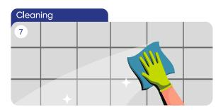
Clean any excess adhesive from the tile surfaces and grout lines immediately with a damp sponge or cloth.
