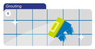
• Grouting should be carried out after 24 hours of tiling. It is advisable to use the appropriate grouting material from Magicrete range of cementitious or epoxy grouts.
